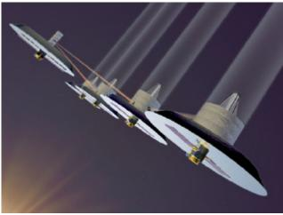
The Terrestrial Planet Finder will be a space interferometer. One possible design would use four space telescopes flying in formation, beaming their images to a fifth combiner spacecraft.
